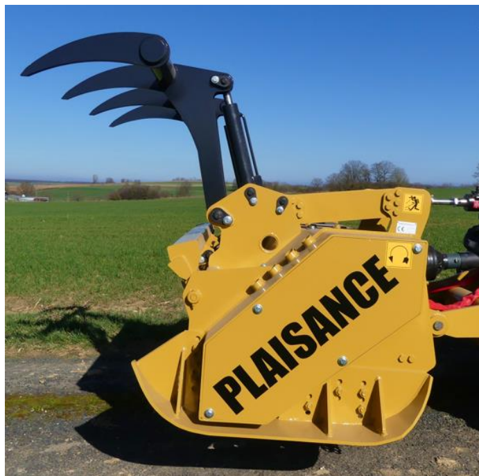
Rakes raised – Door opened
