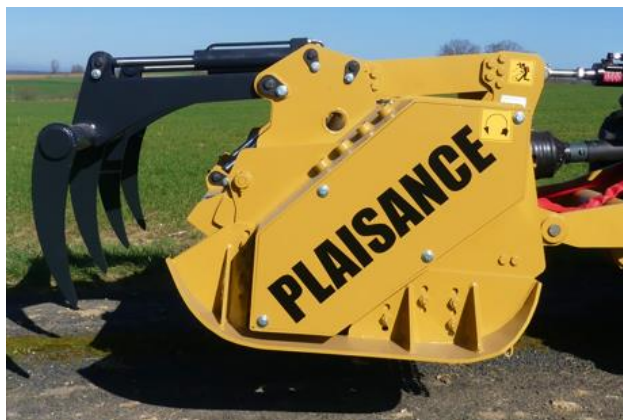
Rakes lowered – Door closed
