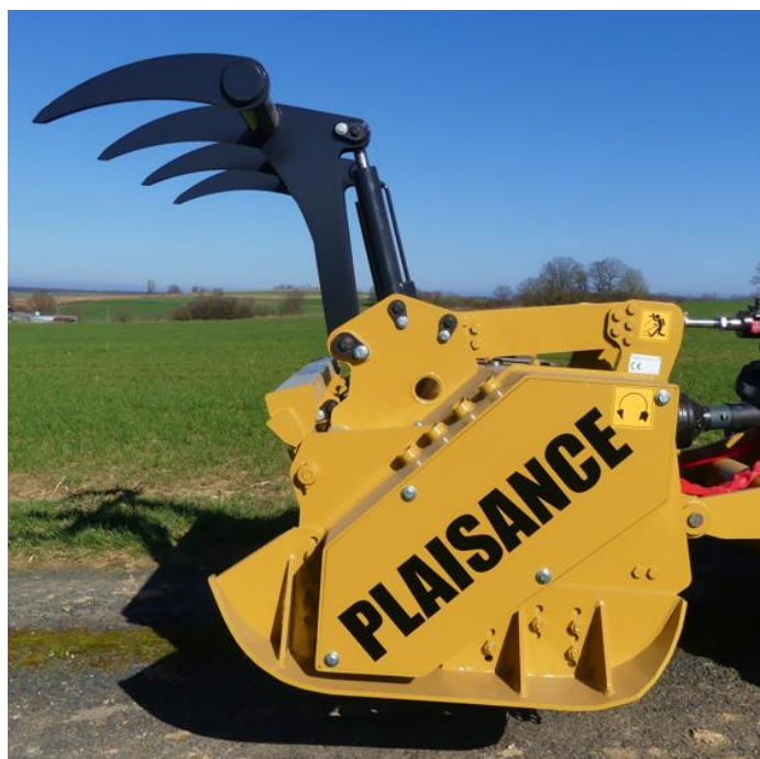
Rakes raised – Door opened
