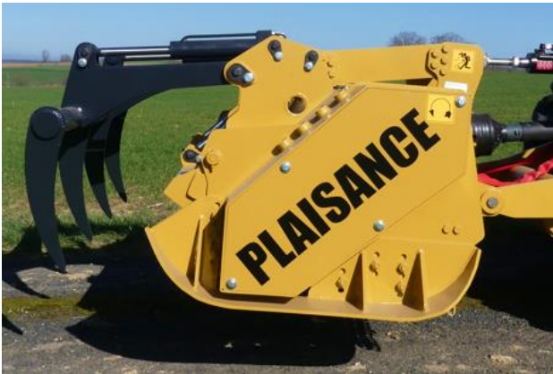
Rakes lowered – Door closed
