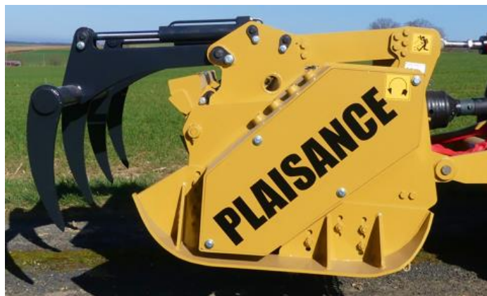
Rakes lowered – Door opened
